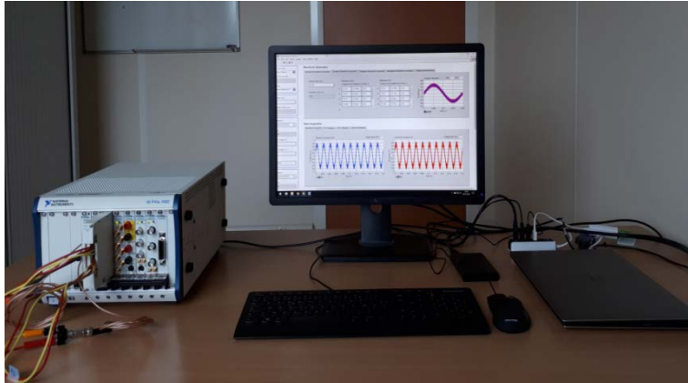
Figure 6 LNE waveform platform for supraharmonics generation and acquisitions
